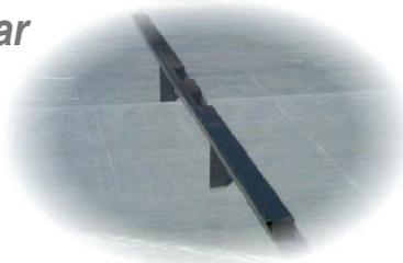
The special guide bar, which replaces the standard 40mm rubber model, is welded to the lift arm providing an arm stop which keeps the platform 80mm from the doors. This leaves sufficient space for the rear door locks for vehicle bodies equipped with doors. Cut outs have been made for the lock bars at floor level. With this special guide bar installed it is not possible to lock the tail lift platform with the standard mechanical locks.
