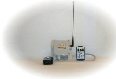
Radio control. Compact and simple to install. The system operating frequency of 433.92Mhz (418MHz in the UK) operating on the FM band is subject to far less interference and hence better function reliability than previous systems. Approved in Austria, Belgium, Canada, Czech Republic, Denmark, Finland, France, Germany, Iceland, Netherlands, Norway, Sweden, Switzerland and United Kingdom. New countries are being added, ask for details if your country is not listed.
